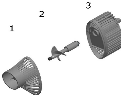
**Fig. 5: Structure NanoProp 5000**
